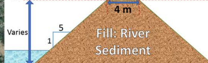
LH Elev. 12.2 m Typical Dyke Cross Section RH Elev. 9.7 m
