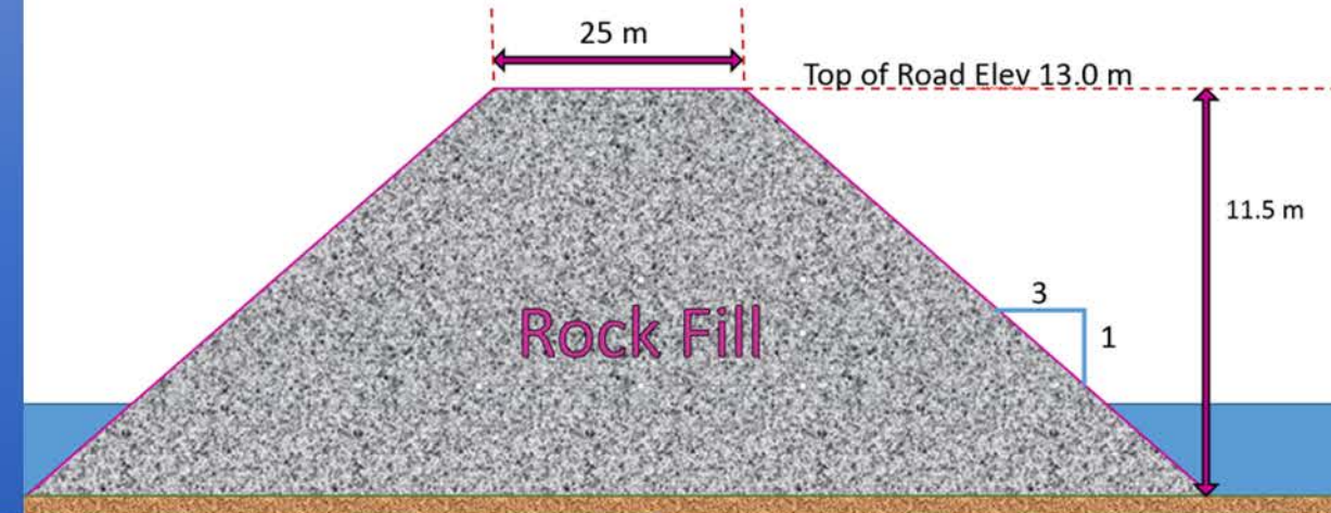
Highway 102 Aboiteau Cross Section
